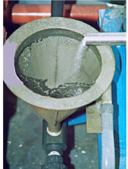
Polymer feed into the Washdown Funnel and being drawn through the Jet Eductor
