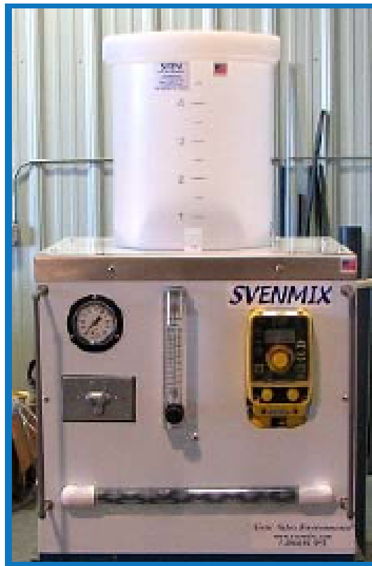
LIQUID POLYMER MIXING SYSTEM
