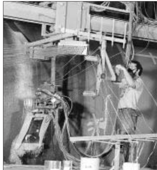
Structural wall is constructed by simultaneous glass chopping, resin spraying and hoop filament winding. (Winding glass is visible at top of photo.)
