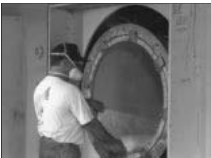
Fiberglass mat is placed into the mold on top of a layer of plain or pigmented mold coat.
