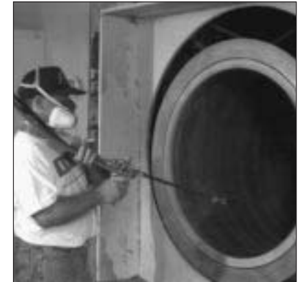
Polyester resin is sprayed onto the mat while the mold cylinder is revolving. This centrifugal action forces the resin through the mat, saturating it.
