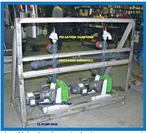
can supply chemical at any point of injection. Properly sized one pump can do the work of two.
