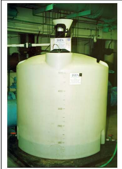
SVENMIX 550 Gal. Graduated Polyethylene Tank and SVENMIX LS ¼ HP Low Speed Mixer with SVENMIX High Turbulence Impeller. This unit is equipped with a top mounted Eductor/Wetting Funnel for mixing Anionic Polymer. The entire unit is mounted on a stand with a pump shelf.
