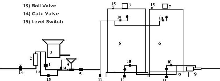
Control Panel will start-up Volumetric Feeder and Solenoid Valve and keep them energized until the level in the tank closes the level switch. This will shut down the Solenoid Valve and Feeder and close the Isolation Valve on the tank just filled and open the valve on the other tank. Isolation Valves can be manual depending upon how much manual control is required.
