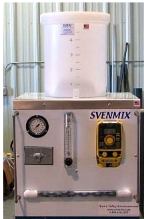
LIQUID POLYMER MIXING SYSTEM
